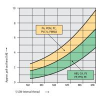
All table values apply only if the screw is inserted to at least 50% of its length in the threaded insert.
